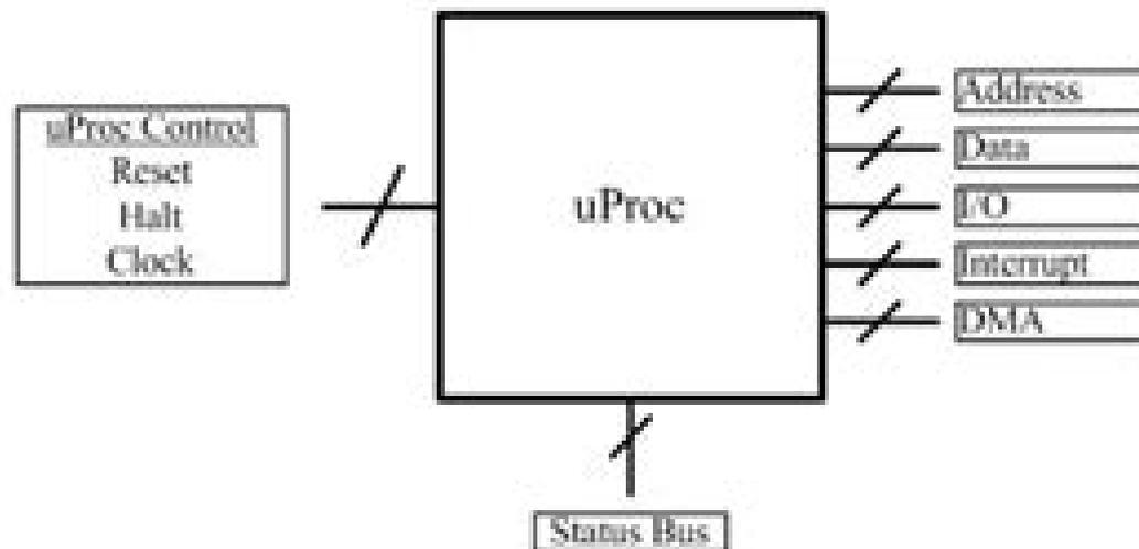
5 Components of a  $\mu$ computer system
